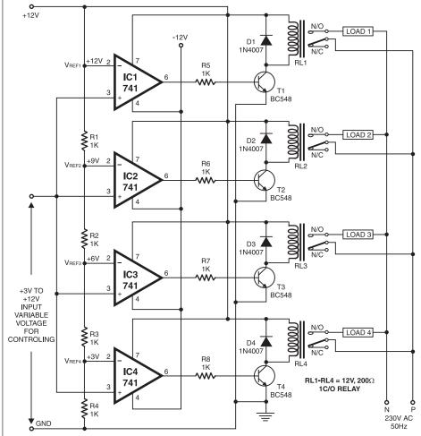
age input terminal; for example, relay RL4 energises when controlling voltage input of + 3V is available at non-inverting pin 3 of IC4. Four electrical equipment can be
